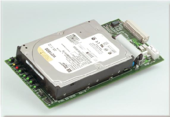
Each EtherDrive® Storage Blade connects to a port on an Ethernet network. Host systems query for an available blade and reserve it. The storage appears as a local disk drive. No hard-to-learn storage management applications. Just a few simple Linux/UNIX commands supplied with the AoE driver.
